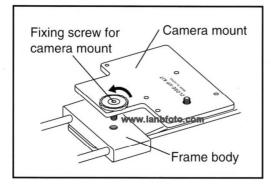
1. Remove the camera mount from the frame body.
