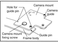
**5.** Set the camera mount according to the guide pin of the frame body and fix.
